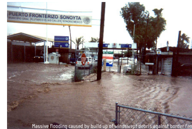
Massive flooding caused by build up of windwept debris against border fence
